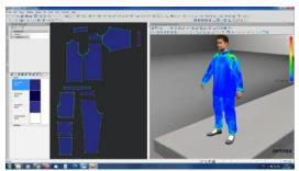
*Fig3*: Simulation of the PPE system for intervention in emergency situations that integrates the inner layer (in contact with the skin) - Underwear PPE and the intermediate layer (base) – Duty uniform
