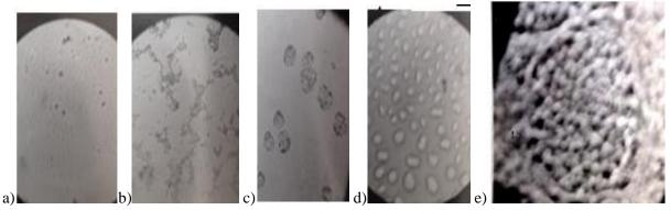
**Fig.2**: Optical microscopy images (1000x) for samples: a)**4**- mezzo and microelements; b)**2**-Gemini surfactant; c)**3**-Bola surfactant; d)**4**-collagen gelatin with mezzo and microelements +surfactant Gemini; e)**5**- collagen gelatin with mezzo and microelements +surfactant Bola
