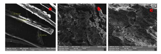
Fig. 4: SEM micrographs of untreated immature coconut fibers
