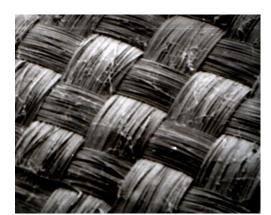
Fig. 3: Electron microscopy images for the obtained fabric (40X magnification)
