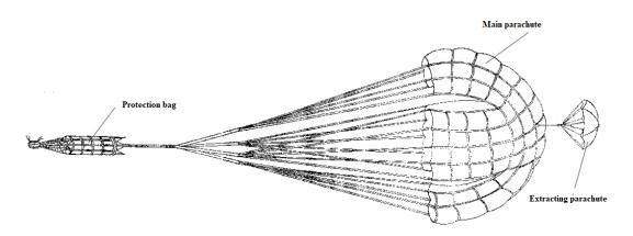
Fig. 2: Diagram of the braking parachute assembly
