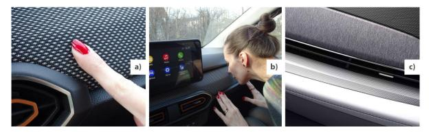
Fig. 2: a) Padded textile insertion (Dacia Sandero Stepway 3); b) Simulation frontal accident -the padded area ensures frontal protection to passengers; c) Padded textile insertion applied on the dashboard of Ford Mustang Mach – E 2021vehicles
