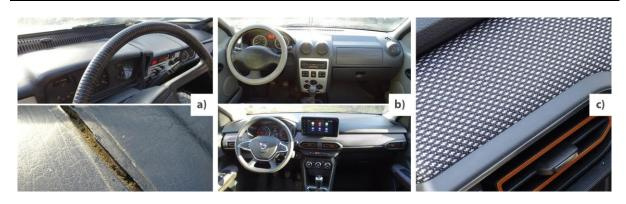
**Fig. 1:** a) Dacia 1310 dashboard made of polyurethane and PVC foil - damage caused by the overheating of the material during summertime; b) Comparison between a conventional ABS and PVC dashboard (Dacia Logan 1) and an ABS and PVC dashboard with a fabric insertion (Dacia Sandero Stepway 3); c) Fabric insertion - detail (Dacia Sandero Stepway 3)
