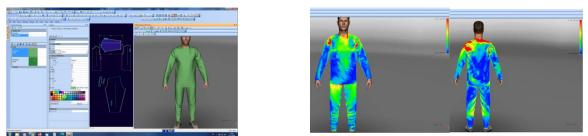
Fig. 1: Inner layer simulation - underwear PPE: Suit consisting of long-sleeved blouse and long pants
