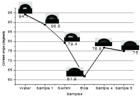
Fig. 4: The contact angle measurements results for samples 1- collagen gelatin with mezzo and microelements,
